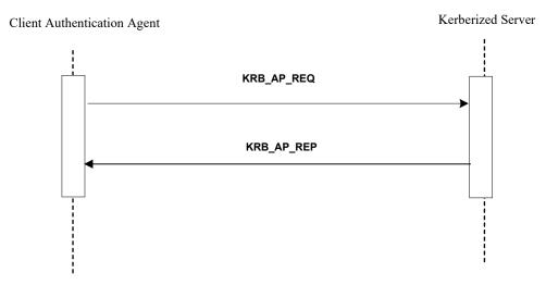
Figure 3.4-1: Kerberized Communications
